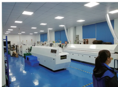
2 SMT lines 1 wave soldering line
